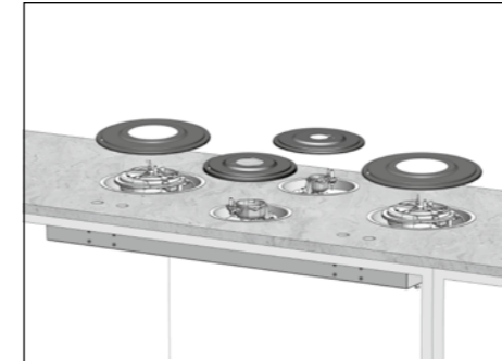
7. Position the heat shields, with the sealing rings in place (step 2), onto the burners and screw them into position with the screws provided.
