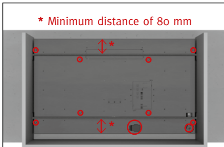
4. Position the support bar in such a way that the mounting screws, gas connection and the electrical connections remain free and accessible.
